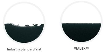
2 ml - Cross Section WFI autoclaved for 4 hrs at 121°C (x20 k)
